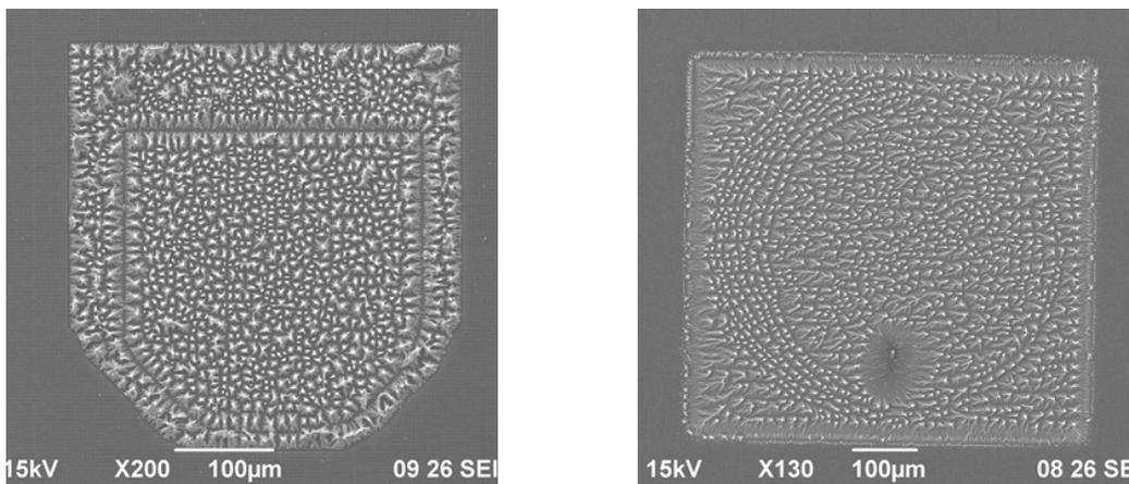
Fig. 5. Scanning electron microscope images of the footprints of wetted area for samples with the same microstructures but different stiffness (a) 1000 MPa (b) 600 MPa.
