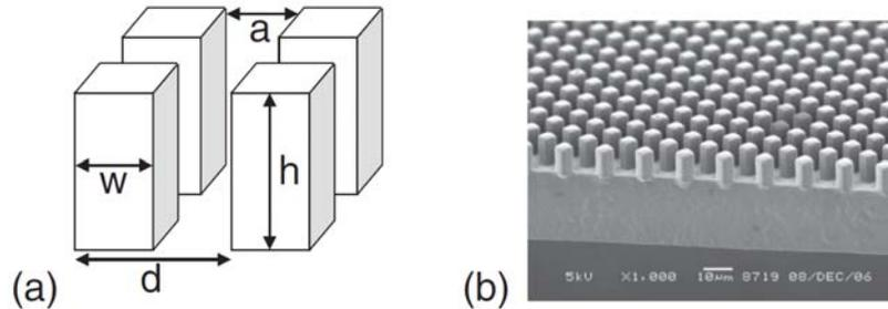
Fig. 2. Sketch and (a) and scanning electron microscope image (b) of the micropatterned substrate [1].
