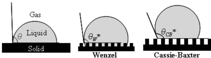
Fig. 1. Schematic diagrams of droplets sitting on surfaces with different wetting behaviors [5].
