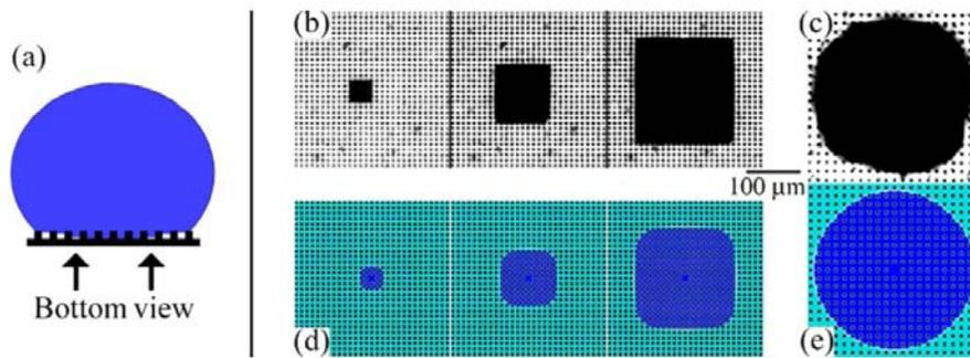
Fig. 4. Bottom views of the front evolution of the transition, as sketched in (a). (b) Three snapshots for the case with  $a = 5 \mu\text{m}$ . (c) When  $a = 11 \mu\text{m}$ , it resulted in a circular wetted area. (d) and (e) show the results of the corresponding numerical simulations [1].
