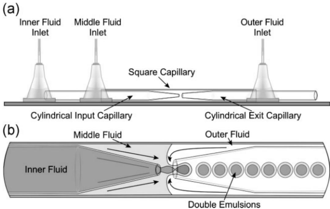
*Figure 1.* Schematic illustrations of (a) microcapillary device and (b) the region of the device where the input and exit capillaries meet. Note that the middle and outer fluids flow in opposite directions within the gap between the round and square capillaries while the inner fluid flows from the interior of the input capillary. Drops are formed and collected in the exit capillary.
